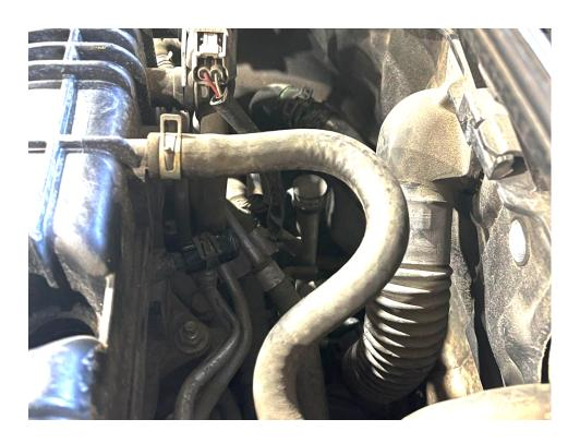
11. Unscrew the stock PCV valve and thread the VQ PCV to -8AN adapter into its place on the passenger valve cover and tighten it down snugly. Make sure you oil the o-ring to make sure it goes in and doesn't catch or tear. (it can help to remove the intake coupler for the next few steps but is not strictly necessary)
