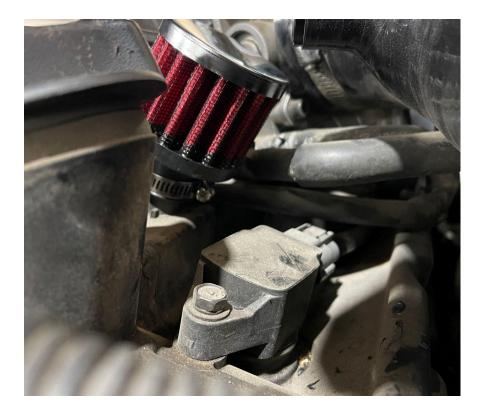
5. Install the 1/2in Vibrant filter onto the Vibrant 90 degree fitting and tighten the clamp.
