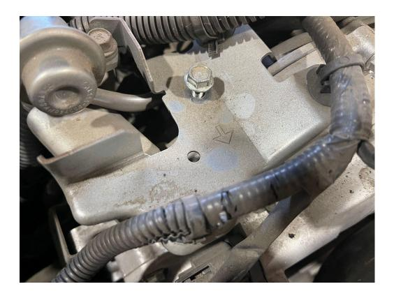
7. Loosen and remove the 12mm M8 bolt on the fuel line bracket on the top of the passenger side of the front timing cover. (underneath the bracket we just moved aside)
