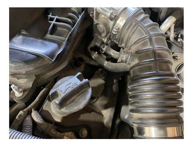
4. Install the 5/8in Vibrant filter onto the open port on the valve cover and tighten its clamp.
