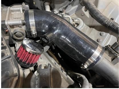
17. Make sure all of your clamps are tight and all of the open ports have been covered by a filter, cap or plug where appropriate. Reinstall your engine cover.
